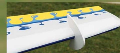
Unique leading edge and generous side force generators allow the Glamour to "defy the force of gravity".
